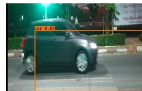
Figure 11. Deep Learning A.I. with YOLO model predict car detection.
