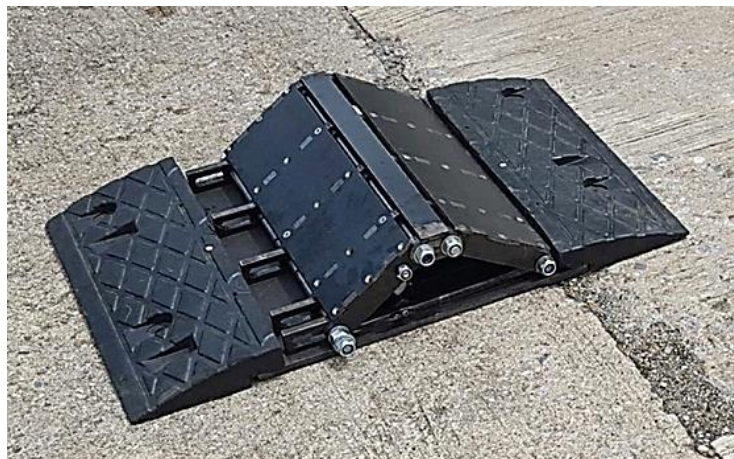
Figure 10: A prototype speed sensitive collapsible mechanical speed bump version V.
