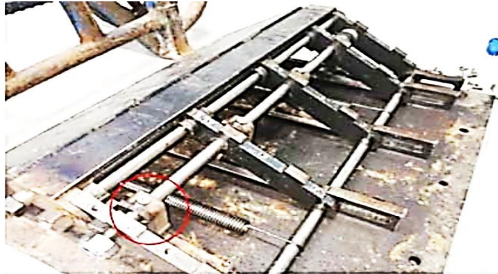
Figure 9: Locking mechanism fixed to a pivot pin.
